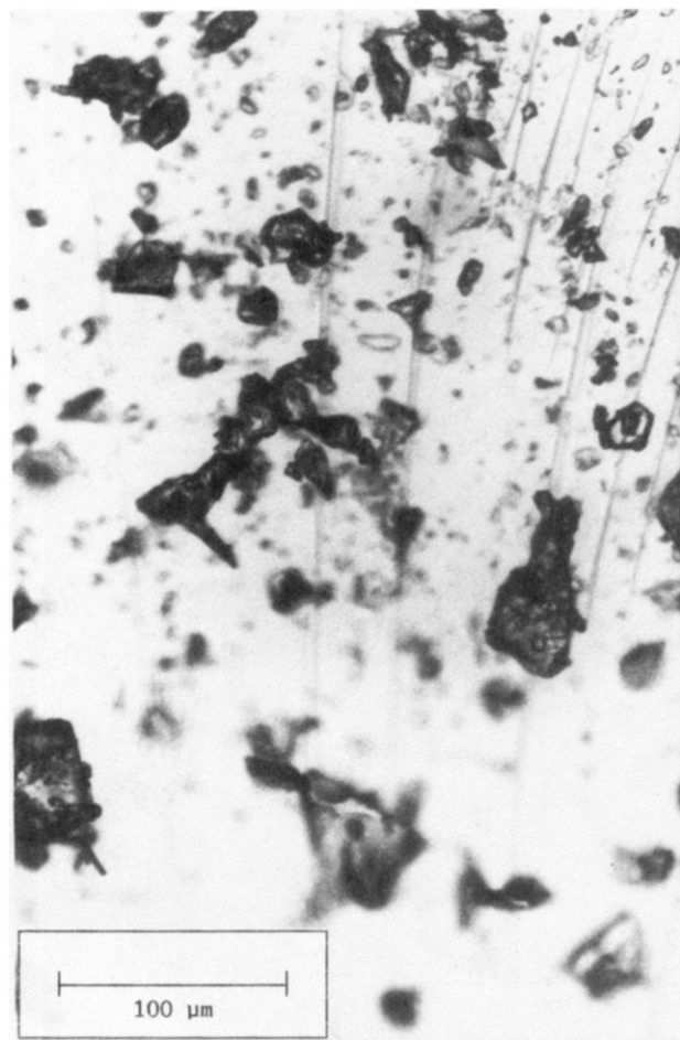
Figure 7. Photograph at nominally 95\times showing the Petpps as received.
